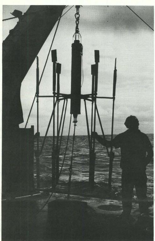
CORROSION EXPERIMENT ready to spend a few months on the ocean floor. Metal samples at top and bottom will allow comparison of corrosion rates from sea water vs. sediment. Except for anchor (block near bottom) entire unit is retrievable on command.
